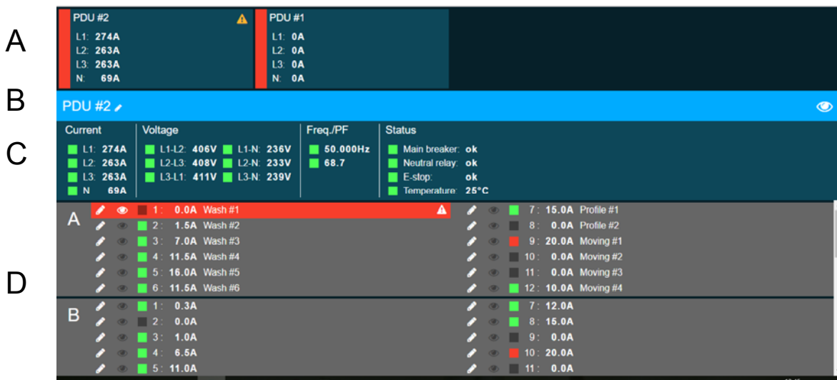
Figure 6. Remote monitoring – main window
